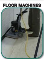
**TOMCAT'S EDGE** Series of surface preparation machines gives operators the ability to remove multiple layers of finish, without using chemicals. As we all push for new ways to increase our protection of the environment, this new approach can help achieve increased productivity and safety. Available in 20", 28" or 32".
